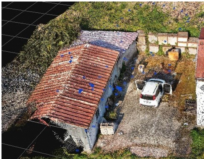
Figure 3. Point cloud calculated by drone images
