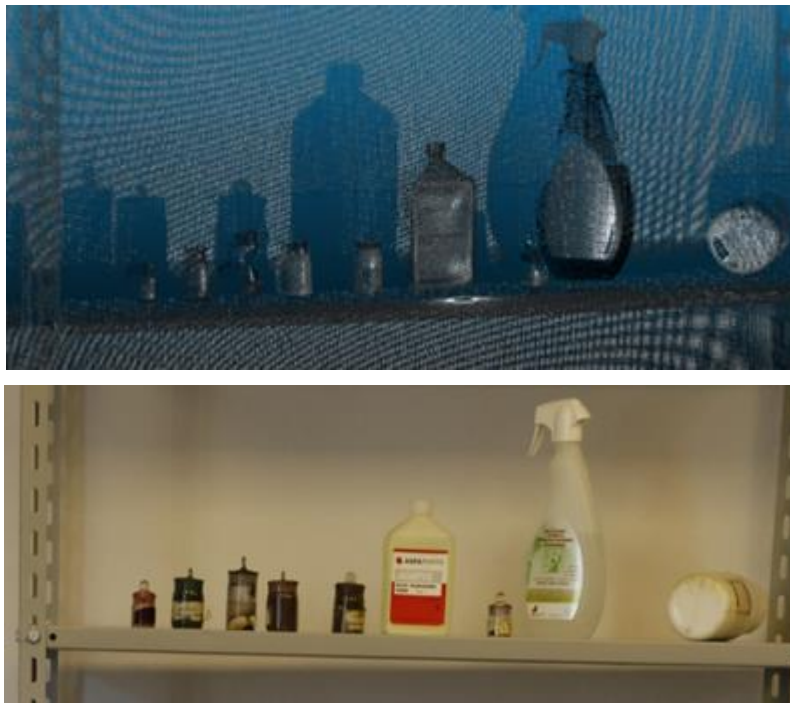
Figure 1. Example of presenting fine details in terrestrial laser scanned models (upper image) and photograph (lower image)
